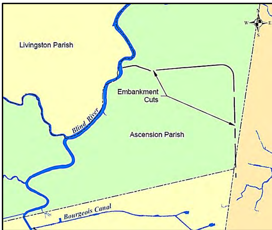
Figure 6.11 – Bayou Secret & Bourgeois Canal Embankment Cuts
