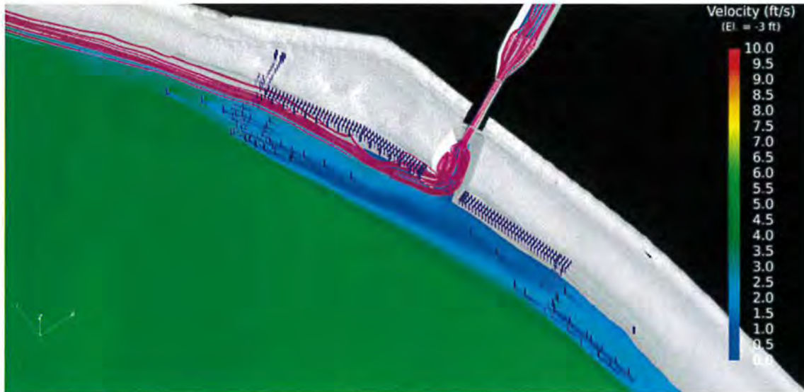
Figure 7 – Velocity contours with streamlines superimposed with Alternative 1 docking facility and operating diversion.
